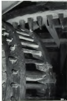
D. The wooden tooth-and-spoke gears required constant maintenance during their more than 100-year (1767-1869) service at the mint.
